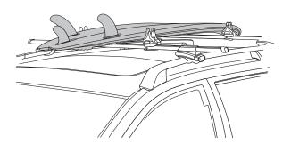
5. Adjust the bases so that the bottom of the surfboard rests on the rubber part of the bases. Tighten all knobs firmly and evenly.
