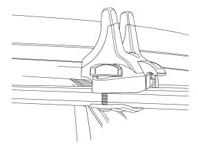
6. Slide the latch on one attachment strap into the clip on a base.
