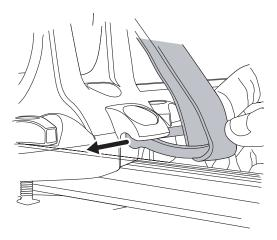
7. Rotate the latch up to lock it into the base. Repeat this step at the other base on the crossbar.
